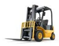
Fig. 1 Counterbalance lift truck
